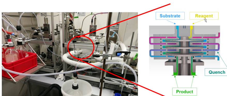
Figure 2. (a) Flowid SpinPro R10 setup for RLi conversions (left) and (b) drawing of SpinPro reactor (right).
